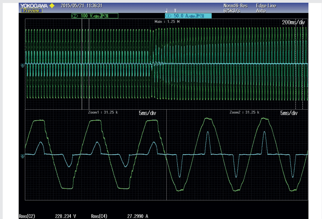
Fig.22. Observation of UPS output waveforms, supplying a non-linear load, during the transfer process from static bypass to inverter. Output voltage distributed to loads on CH2 (green) and loads current demand on CH4 (blue).
